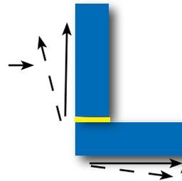
A similar problem can occur with a corner joint, if an indirect force is applied, it can result in the introduction of a cleavage force into the joint.
